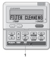
The "FILTER CLEANING" is displayed when the cumulative operation time reaches to the predetermined number of hours in order to notify the time for cleaning.
