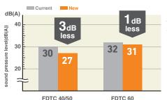
Adopting new turbo fan and improving new heat exchanger enables noise reduction.
