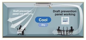
User can position panels by using the remote controller only (RC-EX3A, RCN-T-5AW-E2) when Draft Prevention Panel is available.
