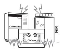
If it is installed near the computer, automatic door, elevator or equipment which generates noise, it will cause to improper operation. Do not install the central control in any area where it is very humid or the vibration is large.
