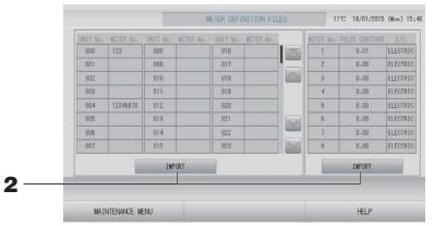
**2.** Insert the USB memory and press the IMPORT button. Select the folder on the Folder Selection screen.
