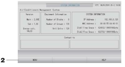
**2.** After checking the content, press the MENU button. It returns to the MENU screen.
