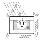
If it is installed in an area exposed to humidity, splashing water or high vibration, it will cause malfunctions. Avoid any place which is exposed to direct sunlight or is near a heat source.
