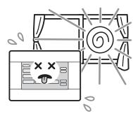
If it is installed under direct sunlight or near a heat source, it will cause malfunctions.
