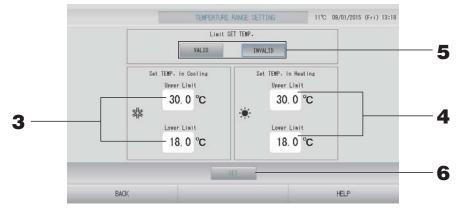
**3.** Press Upper/Lower limit (°C) of SET TEMP. in Cooling. Select temperature by pressing or we button and OK button.
