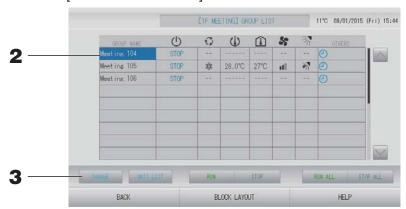
**2. Press the name of the group for which settings or changes are to be made.** The group name is reverse highlighted. To change the page, press the or button.
